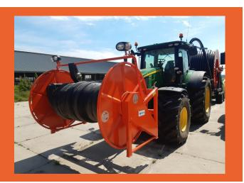
The AP hose reel is developed voor the winding or unwinding of lay-flat hoses for irrigation or drag hose fertilization. The reel is double sided hydraulically driven and provided with a three-point connection. Possibly required front or rear lighting can easily be installed.
